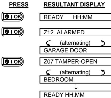
In response to additional clicking of the button, the display shows details of other events retained in open tamper (if any), or reverts to its initial state (see A above).
