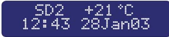
To access the programming menu you must enter the operator's passcode (default 1234). The display shows the first menu option.
