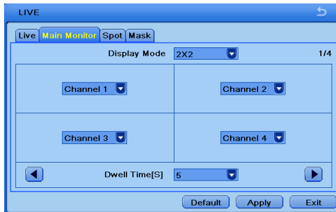
Fig 4-8 Live Configuration-Main Monitor
