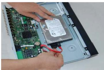
7. Connect the HDD cable and power cable.
