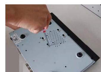
6. Fix the HDD firmly.
