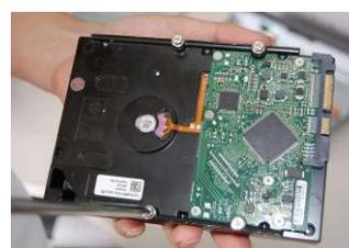
3. Turn four screws for three rounds to fix HDD bracket.
