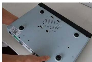
5. Turn the device upside down and then turn the screw in firmly.
