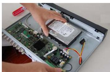
4. Place the HDD in accordance with the four holes.
