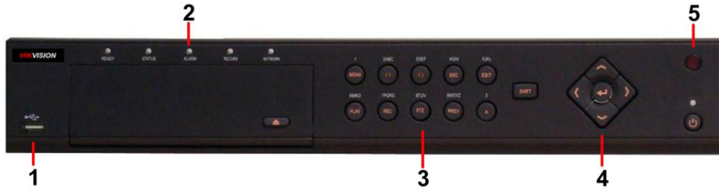
Figure 4. DVR Front Panel Controls
