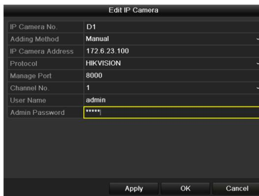
Figure 2. 25 Edit IP Camera Interface - Manual
