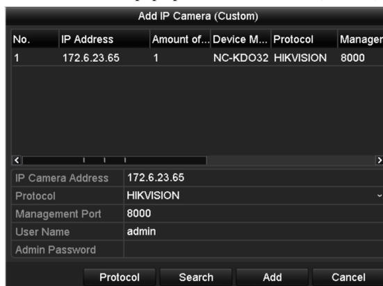
Figure 2. 14 Custom Adding IP Camera Interface
