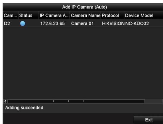
Figure 2. 12 Auto Adding IP Camera Interface
