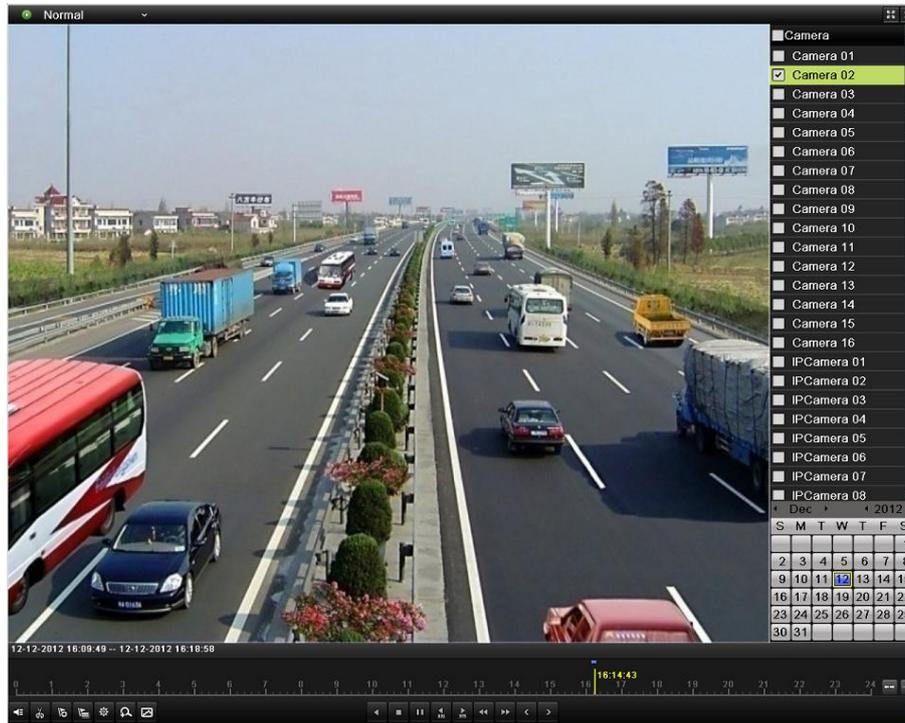
Figure 7. 17 Interface of Playback by Time
