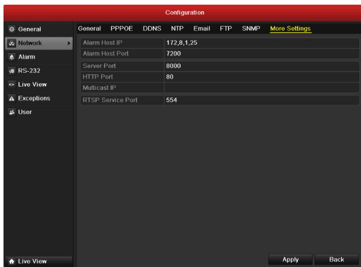
Figure 9.15 Configure Alarm Host
