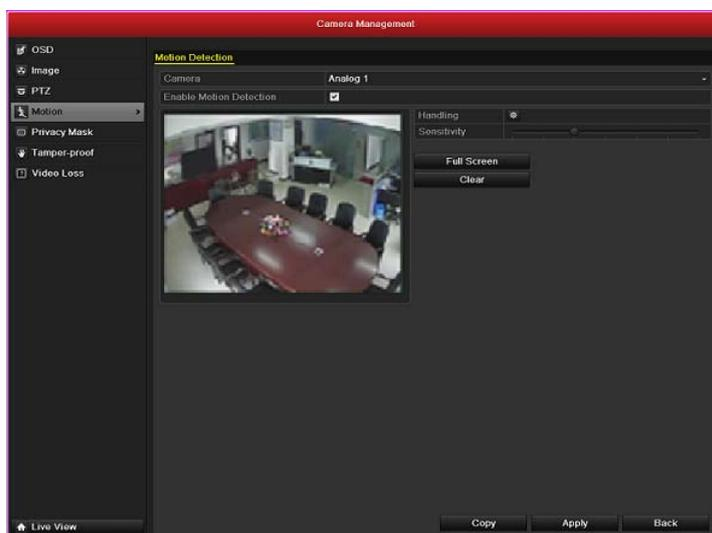
Figure 5.11 Motion Detection
