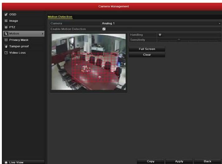
Figure 5.12 Motion Detection- Mask
