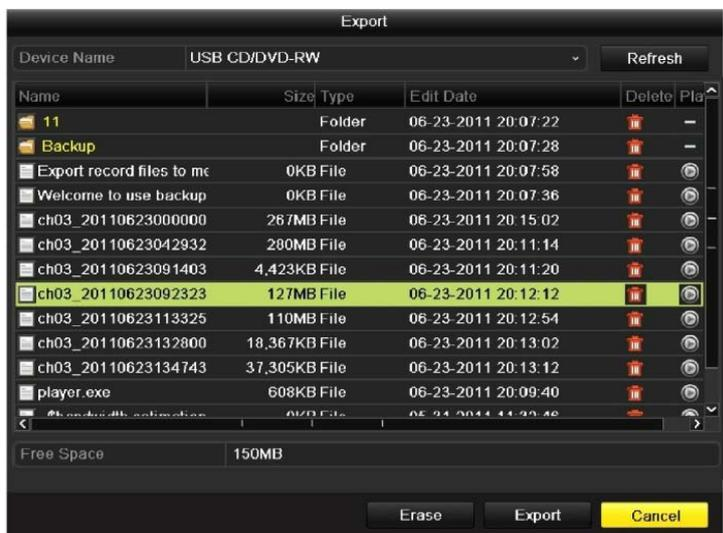
Figure 7.14 Checkup of Export Result using USB Writer
