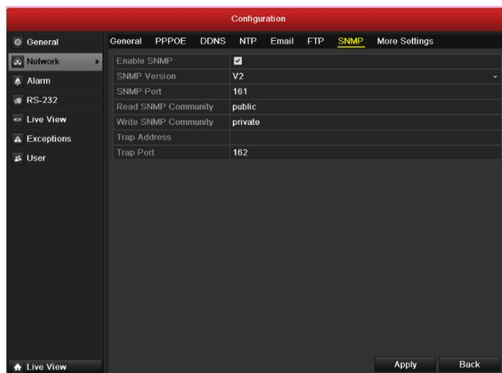
Figure 9.13 Configure SNMP Settings
