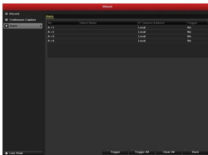
Figure 8.23 Clear or Trigger Alarm Output Manually
