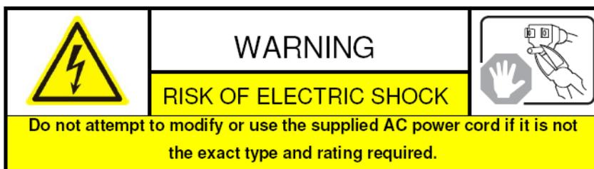
**Power Cord Requirements:** The connector that plugs into the wall outlet must be a grounding-type male plug designed for use in your region. It must have certification marks showing certification by an agency in your region. The connector that plugs into the AC receptacle on the power supply must be an IEC 320, sheet C13, female connector. See the following website for more information <http://kropla.com/electric2.htm>.
