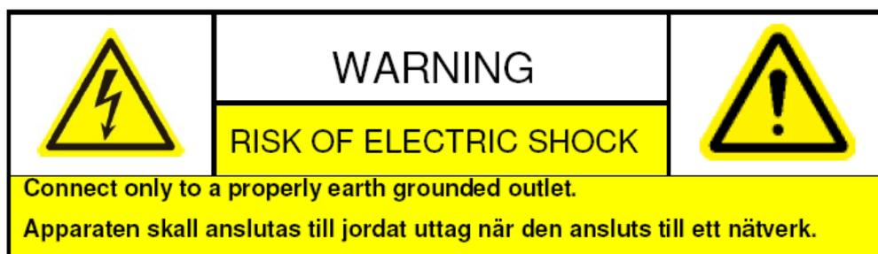
**System Grounding (Earthing):** To avoid shock, ensure that all AC wiring is not exposed and that the earth grounding is maintained. Ensure that any equipment to which this device will be attached is also connected to properly wired grounded receptacles and are approved medical devices.
