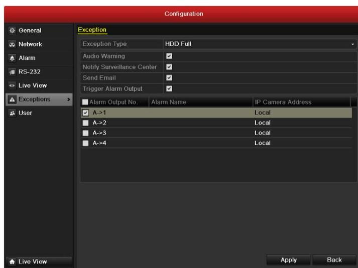
Figure 10.23 Configure HDD Error Alarm
