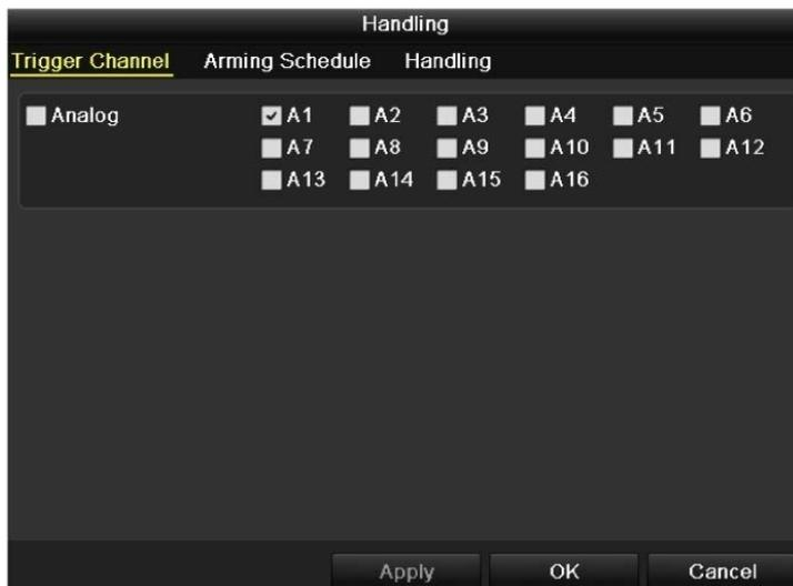
Figure 8.3 Set Trigger Camera of Motion Detection
