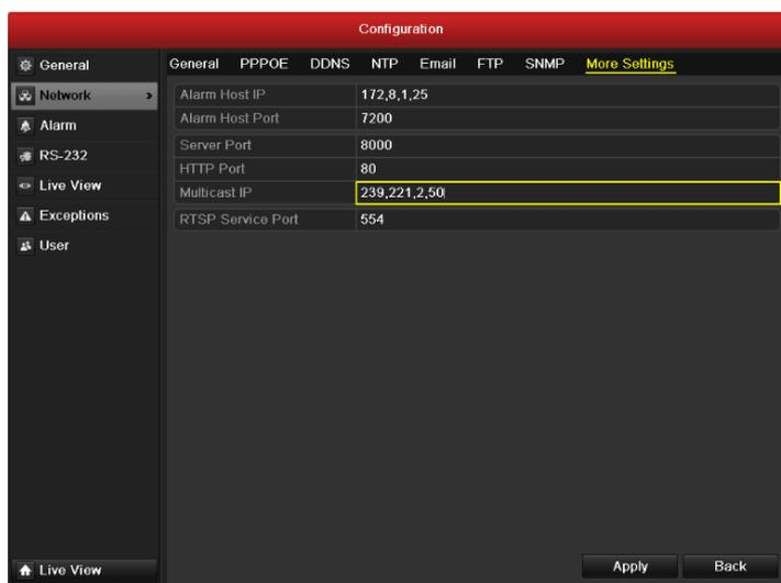
Figure 9.16 Configure Multicast
