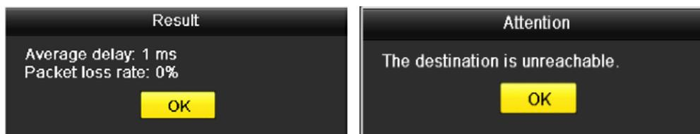
Figure 9.24 Testing Result of Network Delay and Packet Loss
