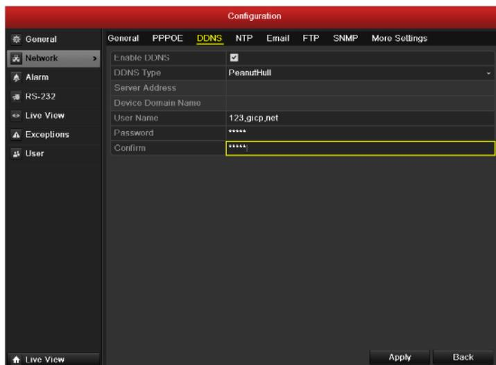
Figure 9.7 Peanut Hull Settings Interface
