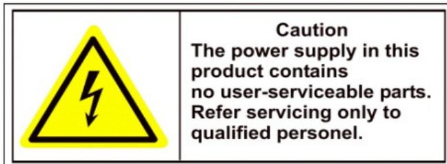
**Power Supply Hazardous Voltage:** AC mains voltages are present within the power supply assembly. This device must be connected to a UL approved, completely enclosed power supply, of the proper rated voltage and current. **No user serviceable parts inside the power supply.**
