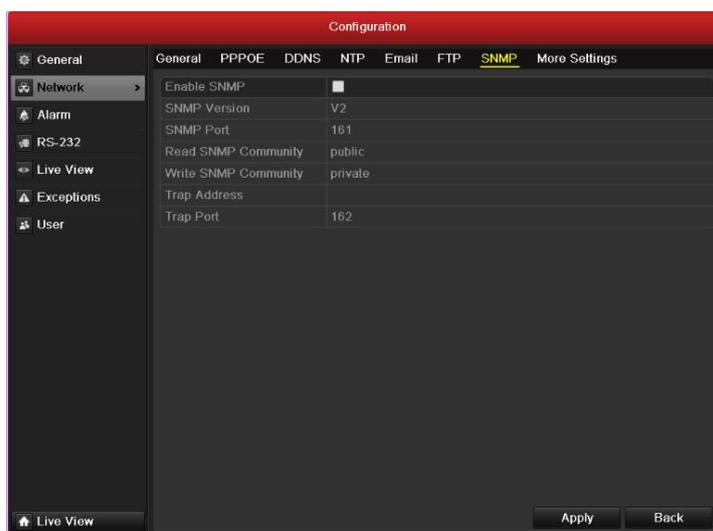
Figure 9.12 SNMP Settings Interface
