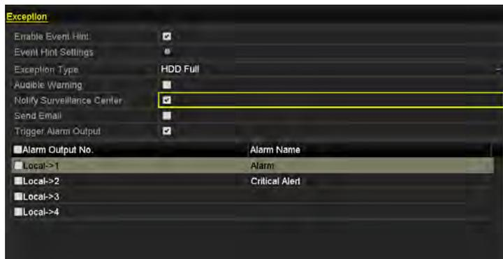
Figure 10. 25 Configure HDD Error Alarm
