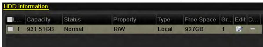
Figure 10. 4 HDD Status Changes to Normal
