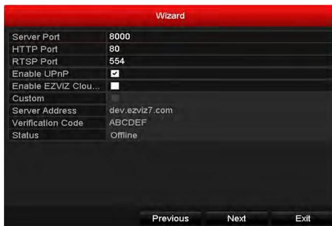
Figure 2. 8 Advanced Network Configuration
