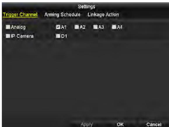
Figure 8.15 Set Triggering Channel of VCA Alarm
