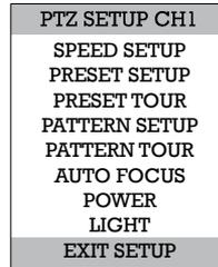
**Speed Setup** – 1-8 [Set the speed that PTZ cameras move.]
