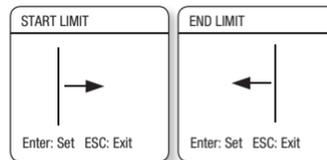
The following picture shows the Tilt Limit setting. Move the joystick left and right to select a movement range from the starting point to the end.
