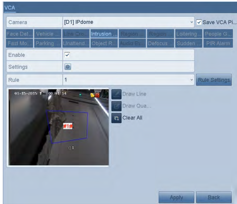
Figure 9. 8 Draw Area for Intrusion Detection
