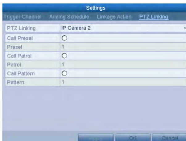
Figure 8. 7 Set PTZ Linking of Alarm Input
