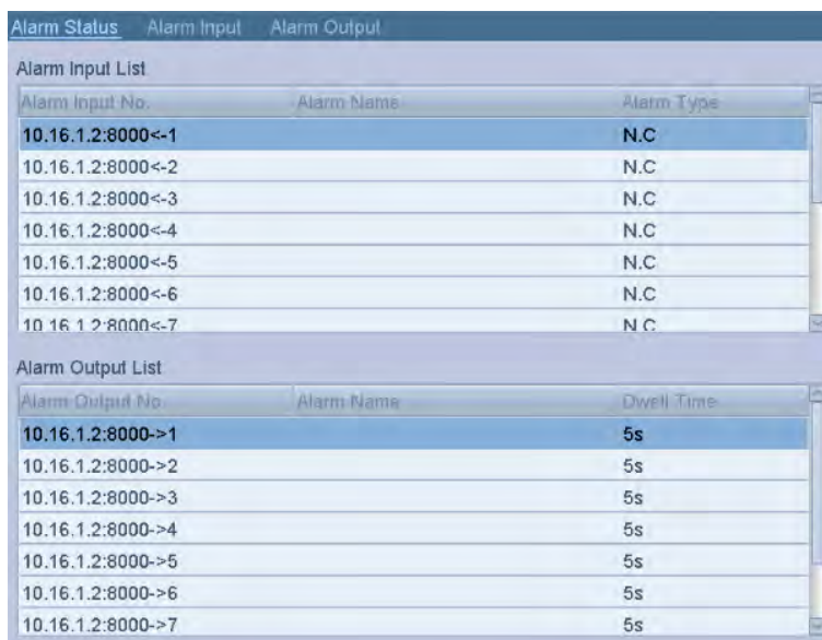
Figure 8. 4 Alarm Status Interface of System Configuration
